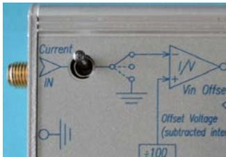
**Grounding sensitive samples by using this input switch is strongly recommended during manipulations on the I/V converter (e.g. changing gain, power on/off).**
