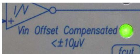
The green LED *Vin Offset Compensated* lights up when the input offset voltage is stabilized within around  $\pm 10 \mu\text{V}$  with respect to the user defined input voltage (up to  $\pm 1 \text{ V}$  given by *Offset Voltage Input*). After power up the device it takes several minutes (up to 30 minutes) until the automatic input offset compensation is completed and the green LED is turned on.
