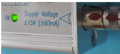
The supply voltage of the LNHS I/V Converter is  $\pm 15$  V with a tolerance of  $\pm 5\%$ . The green LED “ON” lights up when the supply voltage reaches  $\pm 13.5$  V (see left). The typical quiescent current is around  $\pm 40$  mA, but it can rise to  $\pm 60$  mA during normal working conditions.
