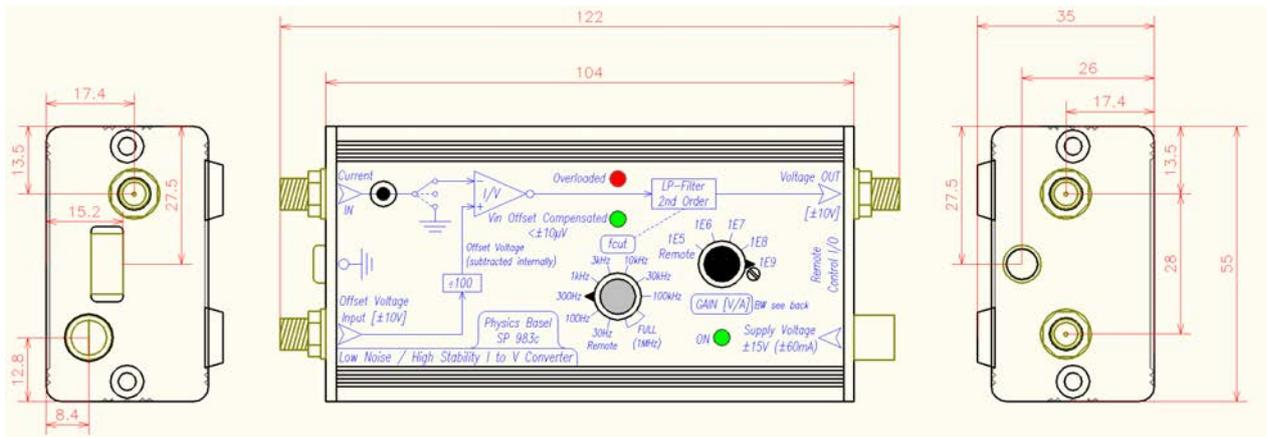
The size [mm] and position of the connectors are shown above. The weight of the device is only 165 g.
