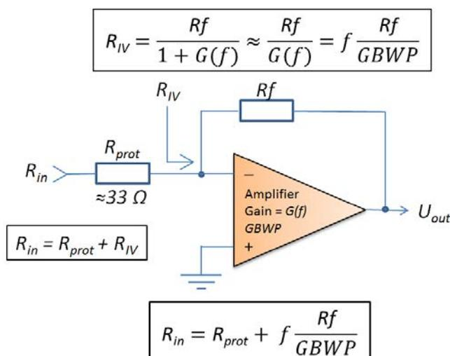
For AC signals the input resistance ( $R_{in}$ ) is increased by the virtual input impedance ( $R_{IV}$ ) of the I/V converter which is depended on the frequency ( $f$ ), the feedback-resistor ( $R_f = \text{gain}$ ) and the gain bandwidth product ( $GBWP$ ) of the amplifier (see left). The  $GBWP$  of the *LNHS I/V Converter* is about 600 MHz.
