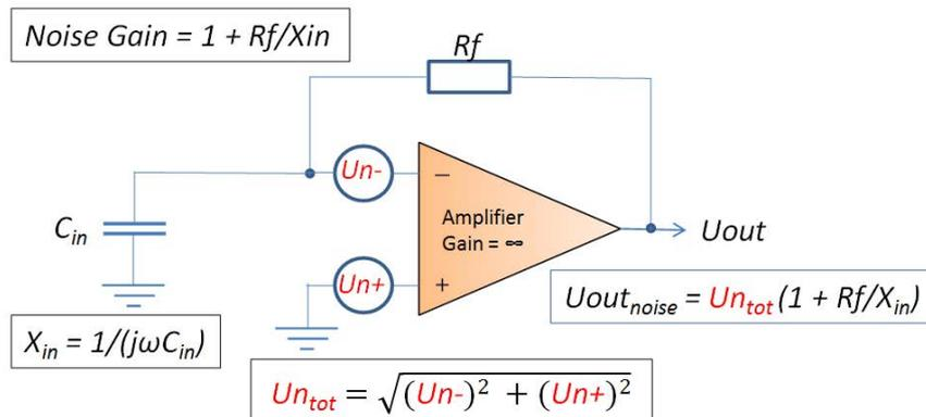
When loading an I/V converter at its input with the impedance ( $X_{in}$ ) the total input voltage noise ( $Un_{tot}$ ) is amplified by the *Noise Gain* =  $1 + Rf/X_{in}$ . Herby the assumption is made that the differential amplifier has an infinite voltage gain.
