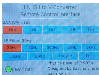
For such installations this *Remote Control Interface (SP 983a)* is a helpful device. It allows controlling the gain and the low-pass filter cut-off frequency remotely and it also displays the status of the *Overload* LED.
