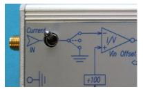
Grounding sensitive samples by using this input switch is strongly recommended during manipulations on the I/V converter (e.g., changing gain, power on/off).
