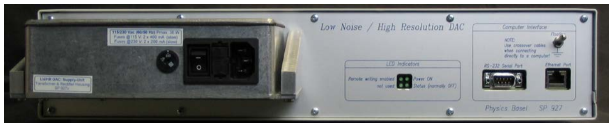
Photo 2: The rear-panel of the LNHR DAC with the attached Transformer & Rectifier Housing on the left. If necessary, this box can be separated from the LNHR DAC up to 4 meters.
