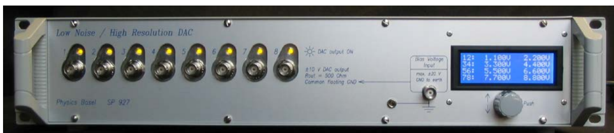
Photo 1: The front-panel of the LNHR DAC with all DAC channel switched on.
