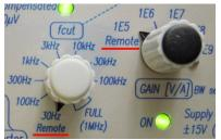
When the gain is remote controlled the rotary switch "GAIN" has to be in the position "1E5, Remote". For remote controlling the LP-filter cut-off frequency the rotary switch "fcut" must be set to the position "30Hz, Remote" (see left). It is possible to control only the gain or only the cut-off frequency remotely and manually set the other by the rotary switch.
